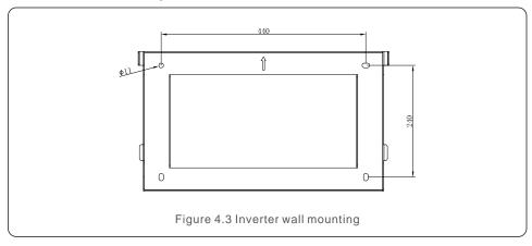
Once a suitable location has be found accordingly to 4.1 using figure 4.3 and figure 4.4 mount the wall bracket to the wall.
