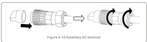
C) Connect AC connector with inverter, then tighten AC connector for clockwise, until hearing a slight clicking sound indicates connection succeed. (see figure 4.16)
