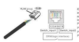
Correspondence between the cables and the stitches of plug, Pin5 and Pin6 of RJ45 terminal is used for the logic interface, other Pins are reserved.
